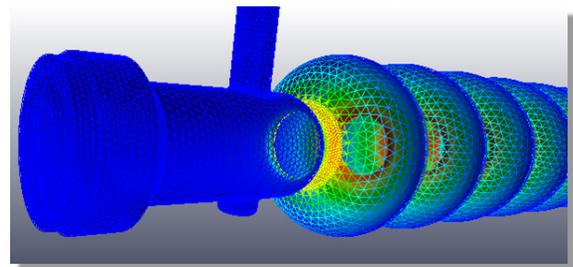
Figure 2: Model of 7-cell coupler region with a short compensation stub diametrically opposing fundamental power port. Mesh coloring corresponds to electric surface field intensity.
