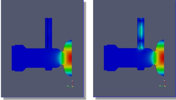
Figure 4: Coupler region of cavity showing fields for two frequencies. Left is on resonance for the 1.3 GHz 7-cell structure and right is obtained by launching a wave through the fundamental power coupler with a frequency 14 kHz higher.
