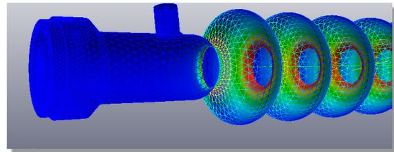
Figure 1: View of 7-cell cavity coupler region of a model without a compensation stub. The mesh coloring corresponds to electric surface field intensity.
