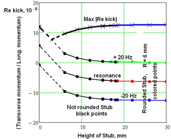
Figure 7: Real part of the normalized coupler kick as a function of compensation stub height. The real part of  $\kappa$  contributes to the transverse kick of the beam. A stub height of zero corresponds to no compensation stub. The  $\pm 20$  Hz values correspond to expected detuning due to microphonics for an operational 7-cell main linac cavity. Top blue line is the worst value of the coupler kick within  $\pm 20$  Hz of the resonant frequency.
