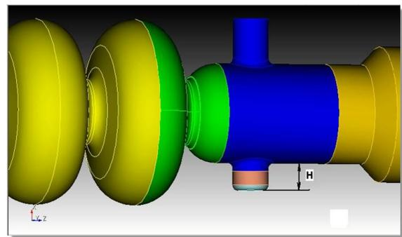
Figure 3: Coupler region of 7-cell cavity geometry. Orange cylinder illustrates method used to tune the compensation stub height, by an additional amount  $H$ .
