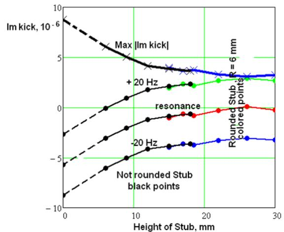
Figure 8: Imaginary part of the normalized coupler kick as a function of compensation stub height. The imaginary component of  $\kappa$  contributes to emittance growth. A stub height of zero corresponds to no compensation stub.
