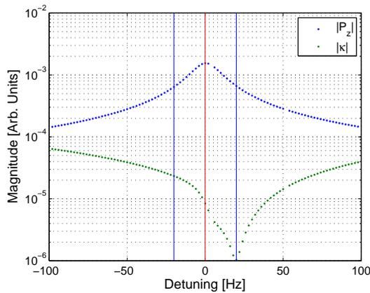
Figure 6: Magnitude of the longitudinal momentum gain and normalized coupler kick versus frequency. The blue lines mark  $\pm 20$  Hz, which is typical detuning operation for the ERL.
