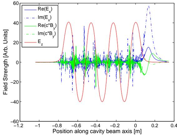
Figure 5: Real and imaginary parts of the field components along the beam axis of the 7-cell cavity. The longitudinal electric field has been scaled down by a factor of 500 for clarity. Note that  $c \cdot B$  is plotted so that the magnetic field effect can be directly compared with the effect of the electric field. The coupler is located at approximately  $z = 0.14$  m, where a small oscillation shows the field interaction with the bunch.
