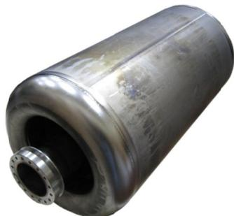
Figure 3: Electron beam welded 112 MHz Nb cavity.
