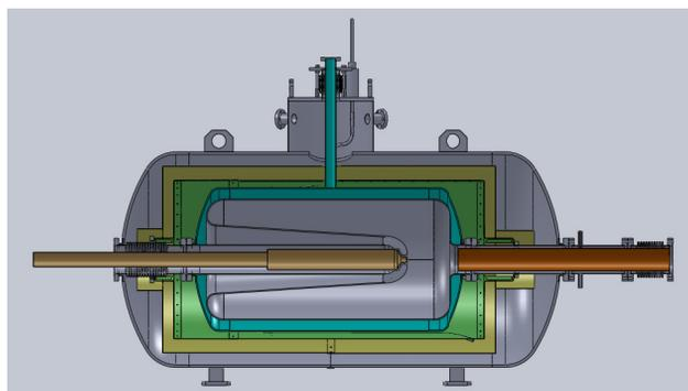
Figure 7: SRF gun cryomodule with the new cathode stalk and FPC.
