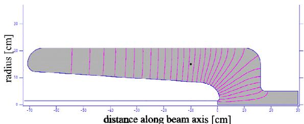
Figure 1: Cavity geometry used in Superfish calculations.
