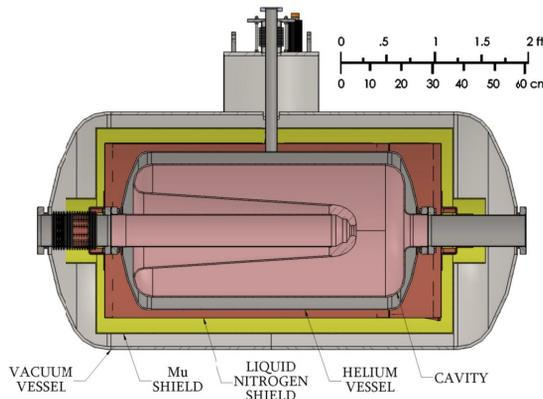
Figure 2: 112 MHz electron gun cryomodule.
