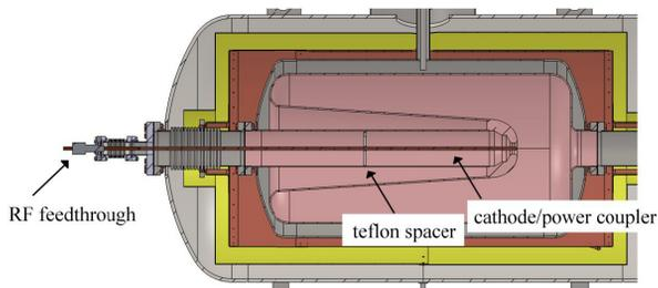
Figure 4: Testing setup for first cryogenic RF test.
