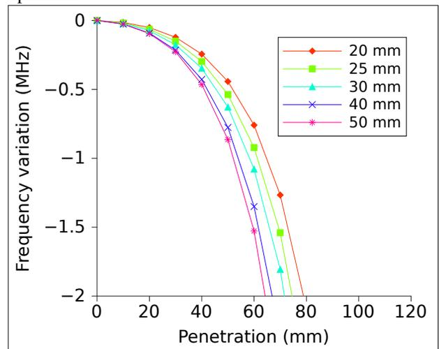
Figure 4. Change of frequency introducing one plunger of perpendicular to a spoke bar, for different plunger radii.
