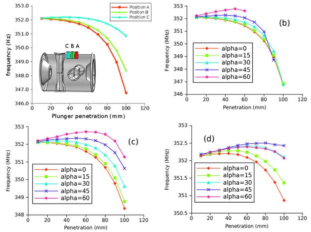
Figure 3: Resonant frequency variation of the cavity (a) when a plunger tuner of 35 mm diameter is inserted in different positions. Frequency change for different azimuthal angles and the longitudinal positions described in (a).
