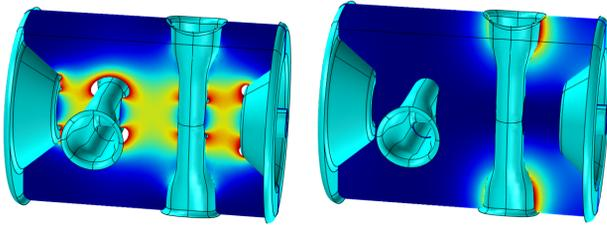
Figure 2. Distribution of electric field energy density (left) and magnetic field energy density (right), with the same colour scale, for the  $\pi$  mode (352.2 MHz) of the cavity.
