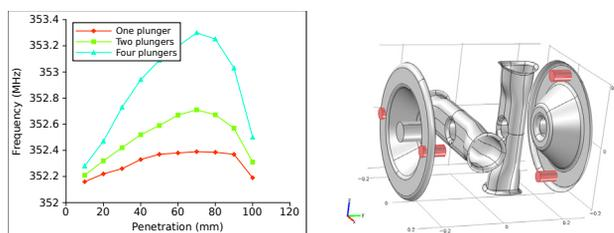
Figure 6: Effect on frequency of introducing plungers through the end covers of the cavity, as depicted in the drawing.
