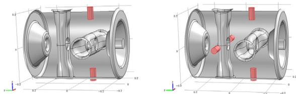
Figure 5. Effect of the number of tuners (of 35 mm diameter) in the cavity frequency. Tuner positions are depicted in the drawings shown.
