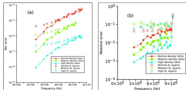
Figure 1: Accuracy of the numerical values of resonant frequencies and magnetic surface fields for a 10 cm radius sphere compared to analytical values. Accuracies are of the same order than the best reported in reference [10].
