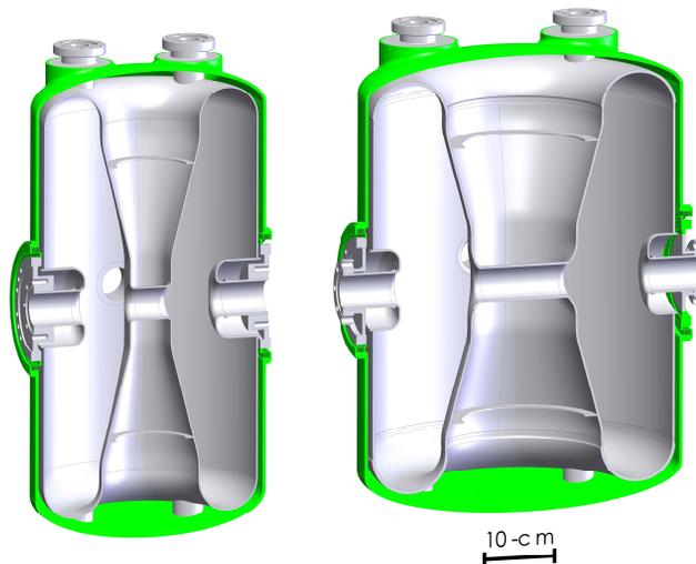
Figure 1: Optimized for production  $\beta = 0.29$  and  $\beta = 0.53$  resonators.
