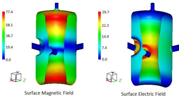
Figure 3: Magnetic and electric field plots.
