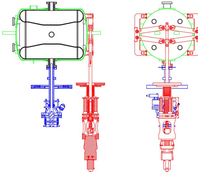
Figure 2:  $\beta = 0.53$  HWR (black), with helium vessel (green), rf coupler (blue) and tuner (red).
