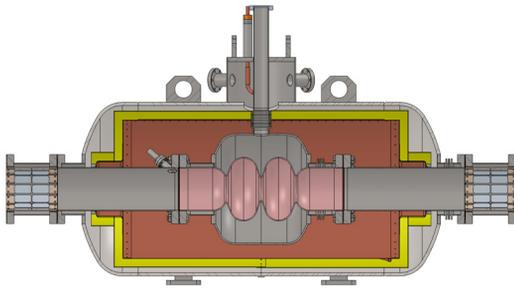
Figure 3: Geometry of NSLS-II 3<sup>rd</sup> harmonic cryomodule.
