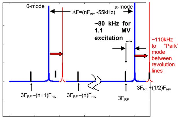
Figure 5: Induced pi-mode voltage as a function of cavity tuning.  $F_{rev} \sim 380$  kHz.
