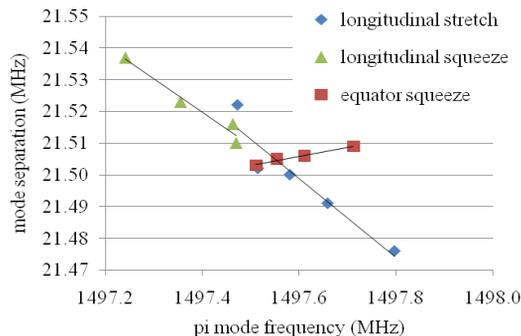
Figure 6: Results of tuning with longitudinal vs. equatorial squeezing, demonstrating frequency adjustment of  $\pi$ -mode and mode separation.
