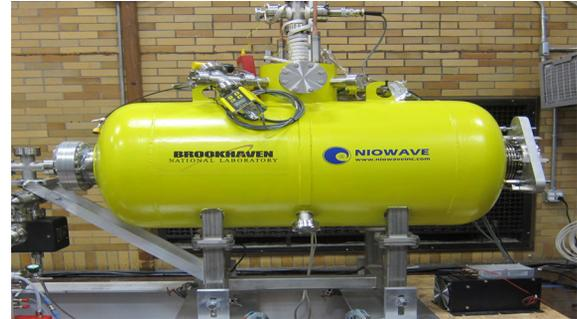
Figure 7: Cold test set up of the 1500MHz cavity.
