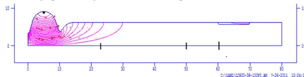
Figure 1: 1500 MHz cavity geometry with Nb-Cu interface (4K), 77K shield and 300K interface marked on axis.
