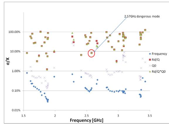
Figure 5: Results of the fabrication error analysis, y axis: standard deviation divided by average value.
