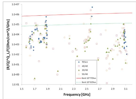
Figure 3: Undamped shunt impedances for various models.
