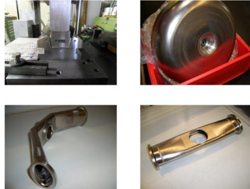
Figure 4: Deep-drawing of a girder component and an end cap of the cavity (top), final welded inclined stem and a straight stem without drift tube (bottom).
