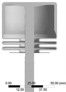
Figure 3: Final design of the 3-cell bellow tuner.
