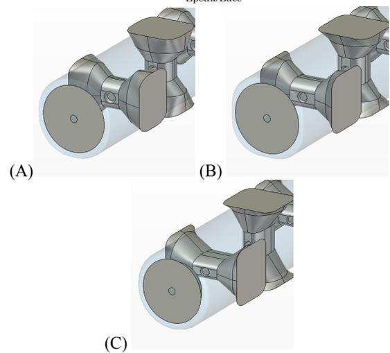
Fig. 5: Typical shapes of spoke cavity near Pareto front of Epeak/Eacc-dominant (A), Hpeak/Eacc-dominant (C) and their medium (B).
