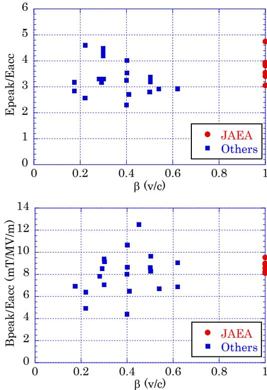
Fig. 6:  $E_{peak}/E_{acc}$  (upper) and  $B_{peak}/E_{acc}$  (lower) as a function of  $\beta$ . Solid circles: our spoke cavity design and solid squares: other spoke cavities shown in references [4-5].
