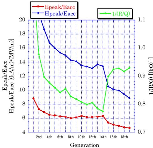
Fig. 3: Average values of Epeak/Eacc, Hpeak/Eacc and 1/(R/Q) in each generation.
