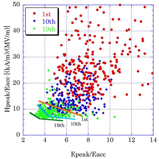
Fig. 4: Distribution (dots) and Pareto fronts (lines) of Epeak/Eacc and Hpeak/Eacc at some generations.
