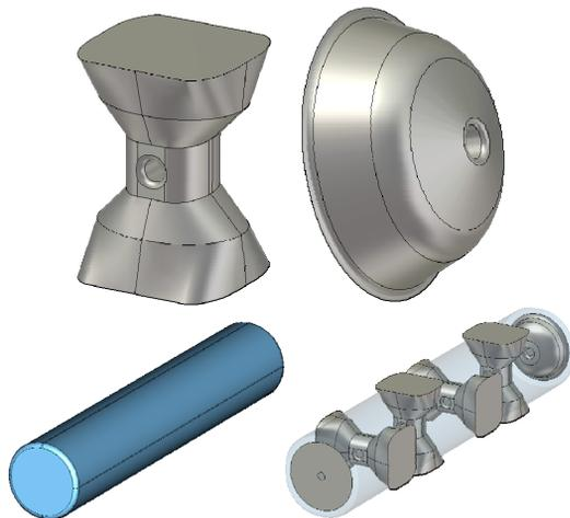
Fig. 2: Example of parts of spoke cavity; spoke (upper left), tank (lower left) and end nose (upper right) and their assembly (lower right).
