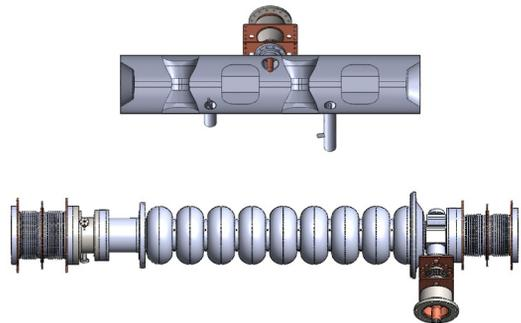
Fig. 1: Schematic views of spoke cavity (upper) and elliptical cavity (lower).
