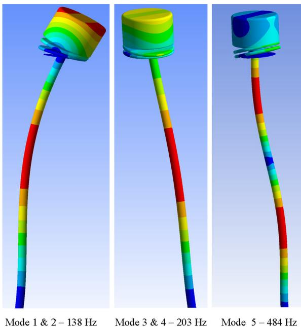
Figure 5: First mechanical eigenmodes of the dynamic bellow tuner.
