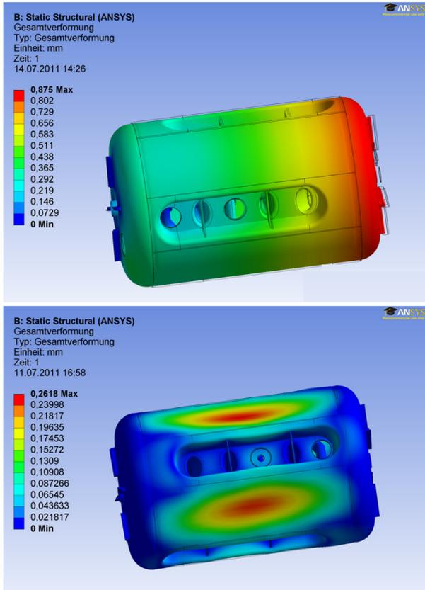
Figure 2: Displacements of the sc 325 MHz CH cavity under Cool-Down (top) and evacuation (bottom).
