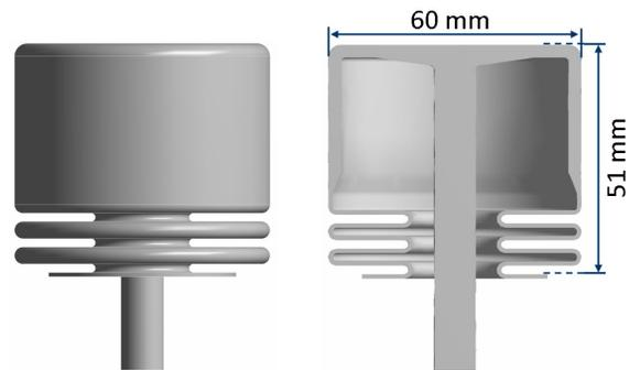
Figure 3: Design of the novel dynamic 3-cell bellow tuner for the sc 325 MHz CH cavity.
