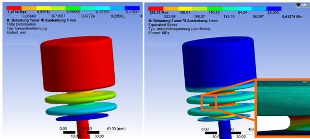
Figure 4: Maximum stroke (left) and max. von-Mises stress (right) of the dynamic bellow tuner.
