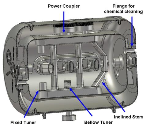
Figure 1: Layout of the sc 325 MHz CH cavity [3].
