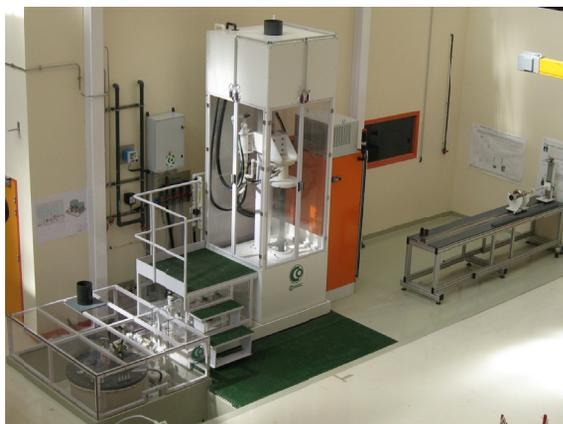
Figure 10: New vertical electro-polishing set-up.
