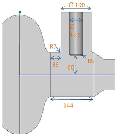
Figure 2: Dimensions of the coupler port (in mm).
