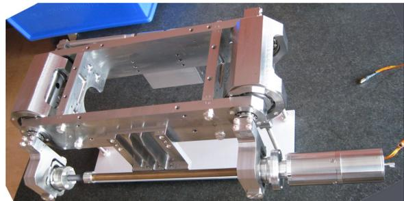
Figure 7: Part of a tuner in preparation of qualification test.
