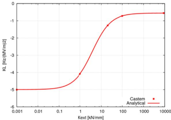
Figure 5:  $K_L$  vs external stiffness  $K_{ext}$ . Analytic curve and points calculated by CASTEM2000.
