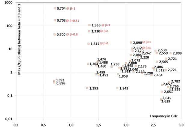
Figure 4: Monopole High Order Modes with frequency and maximal  $r/Q$  for particle  $\beta$ 's between 0.8 and 1.
