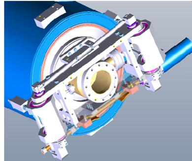
Figure 6: 3D drawing of the tuner on the SPL cavity.
