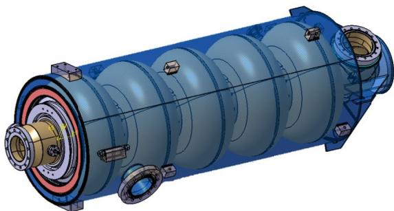
Figure 8: Saclay cavity prototype in its helium tank.
