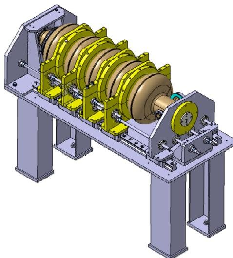
Figure 9: tuning set-up for field flatness achievement at room temperature.
