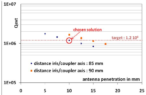
Figure 3: Optimization of the coupler position and the antenna penetration.
