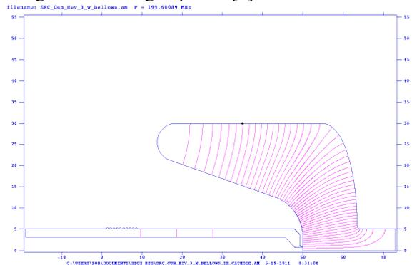
Figure 1: Electromagnetic design showing resonant frequency and final cavity dimensions.
