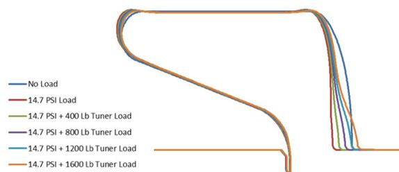
Figure 2: Cavity wall coordinates for different mechanical loads. Distortions shown are exaggerated by 100x.
