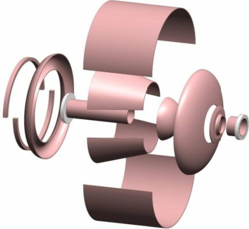
Figure 3: Exploded view showing weld joints.
