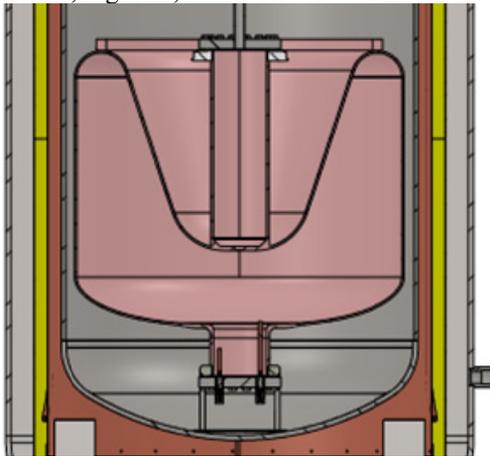
Figure 4: Cavity mounted in dewar with antennae for measuring resonant frequency.
