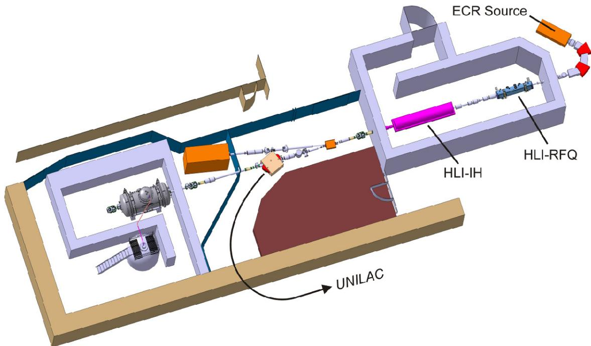
Figure 1: The future layout of the GSI accelerator facility with the cw-LINAC Demonstrator integrated in the existing High Charge Injector (HLI).
