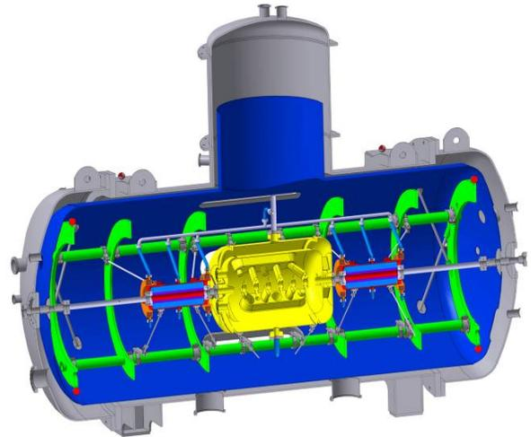
Figure 3: Sectional view of the cryostat. On the top space for a reservoir of liquid helium as well as of liquid nitrogen is reserved.
