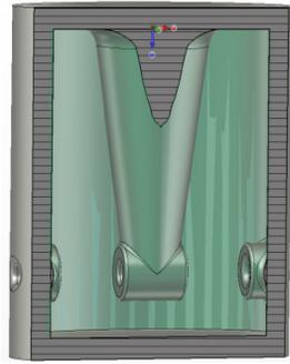
Figure 2: Design of QWR structure.
