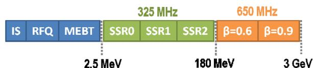
Figure 1: The Project X CW linac.
