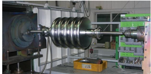
Figure 4: Electron-beam welding of five-cell cavity.
