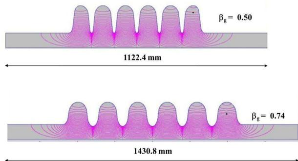
Figure 1: Cavity geometry for PEFP SRF linac.
