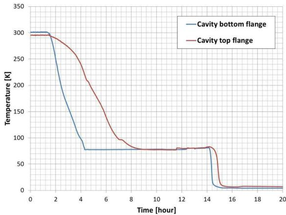
Figure 14: Temperature variation during cooling.
