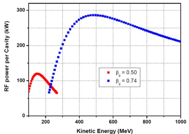
Figure 2: RF power requirement for each cavity.
