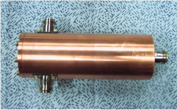
Figure 9: Fabricated split coaxial type RF combiner.
