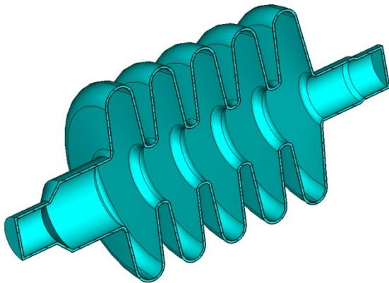
Figure 3: Five-cell prototype cavity.
