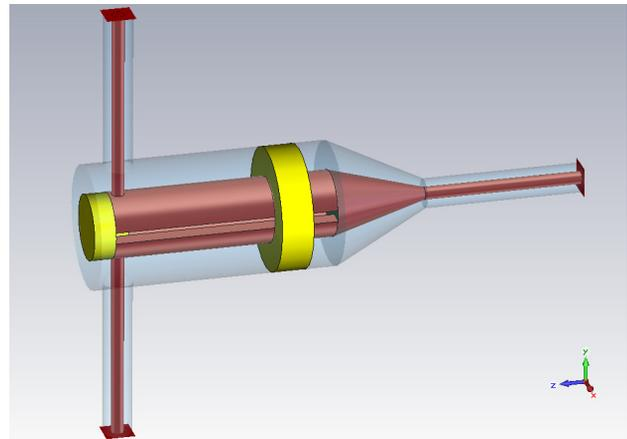
Figure 8: Split coaxial type RF combiner.
