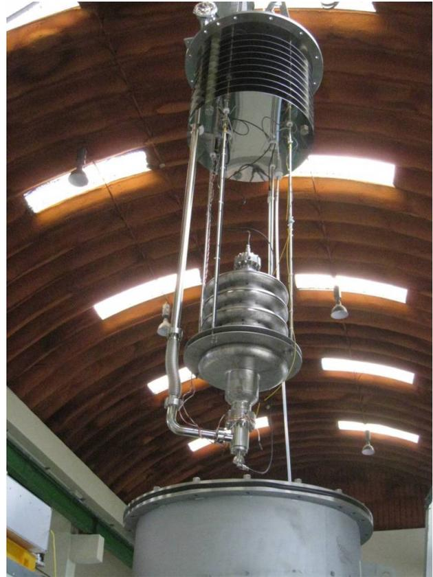
Figure 12: Insert structure with a prototype cavity.
