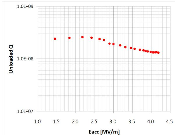
Figure 16: Q0 vs. Eacc for the prototype cavity.
