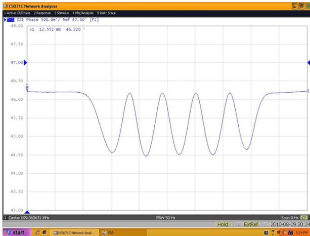
Figure 6: Field distribution after field flatness tuning.
