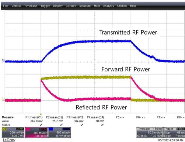
Figure 15: RF pulse waveform during the vertical test.
