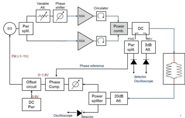
Figure 7: RF System setup for the vertical test.
