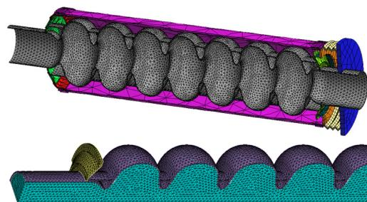
Figure 2: ANSYS Workbench model (top) and APDL model (bottom).
