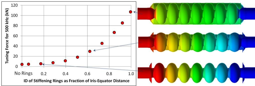
Figure 4: Required force to tune ERL 7-cell by 500 kHz as a function of stiffening ring radius. The images to the right show the location of deformation for three different cases.
