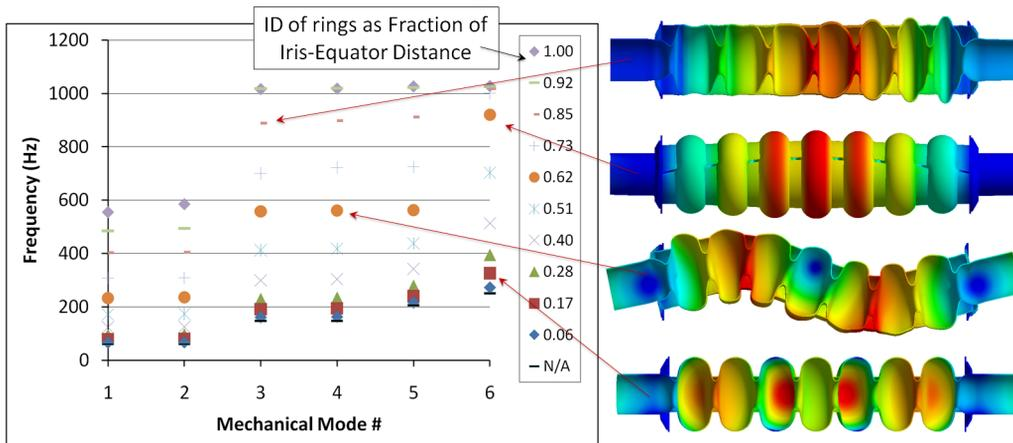
Figure 6: Frequencies of the six lowest mechanical resonant modes of the ERL 7-cell cavity as a function of iris-equator distance.
