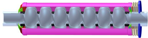
Figure 1: 3-quarter section view of a CAD model of the ERL main linac cavity cryomodule.
