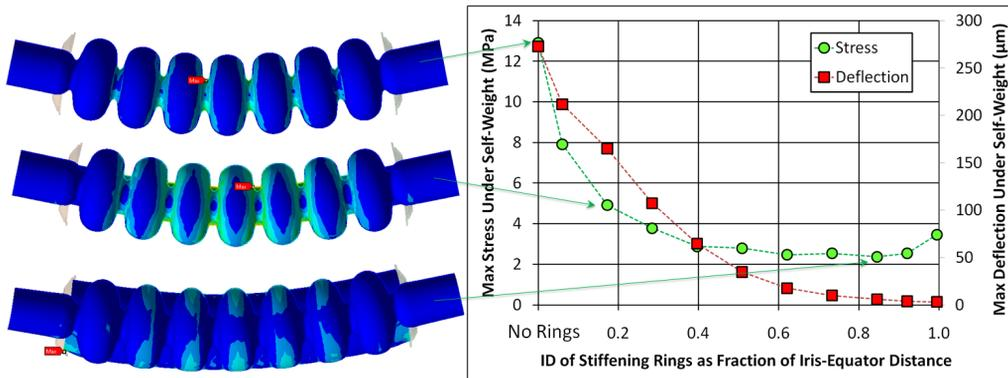
Figure 5: Maximum stress and deflection in the ERL 7-cell cavity as a function of stiffening ring radius when the cavity is resting on its enddisks and deflects under its own weight.
