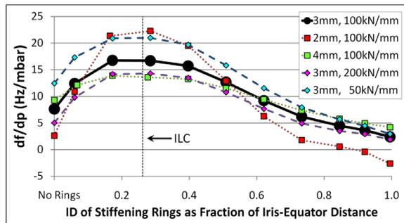
Figure 3:  $df/dp$  in the Cornell ERL 7-cell cavity as a function of stiffening ring radius, wall thickness, and tuner stiffness.
