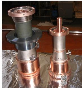
Figure 3: High power input coupler (warm and cold part).
