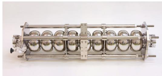
Figure 1: IHEP-01 low-loss large grain 9-cell cavity.
