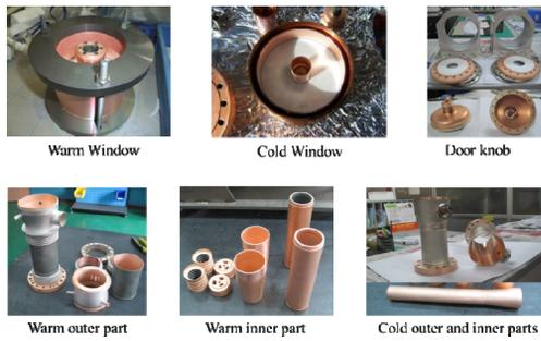
Figure 2: High power input coupler parts.
