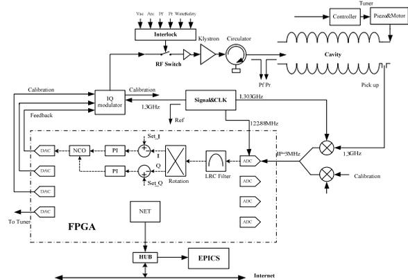
Figure 5: Frame of the digital LLRF test system.
