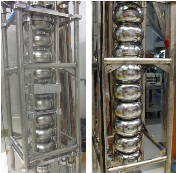
Figure 4: 9-cell cavity testing at JLab under cavity exchange program for ILC cavity R&D. Left: cavity MHI8 from KEK; Right: cavity IHEP-01 from IHEP.
