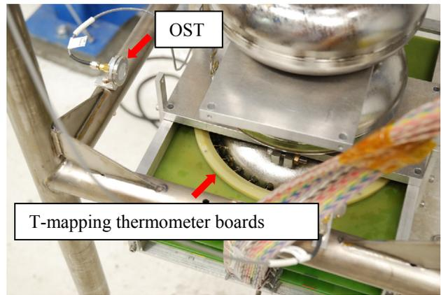
Figure 5: 9-cell cavity quench study instruments: Cornell OST sensors are set-up together with JLab temperature mapping thermometry boards for cross checking.
