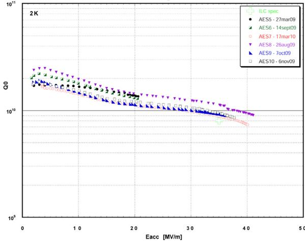
Figure 1:  $Q(E_{acc})$  curves of the six 9-cell cavities of the second AES production batch.
