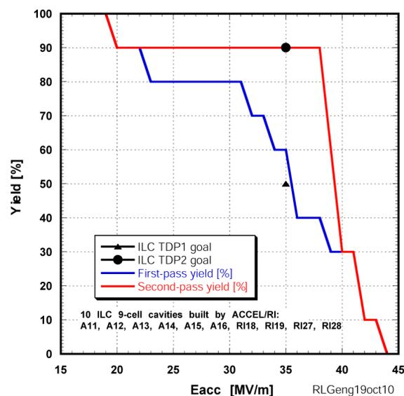
Figure 3: First-pass and second-pass gradient yield based on 10 9-cell ILC baseline cavities manufactured by ACCEL/RI and processed and tested at JLab.
