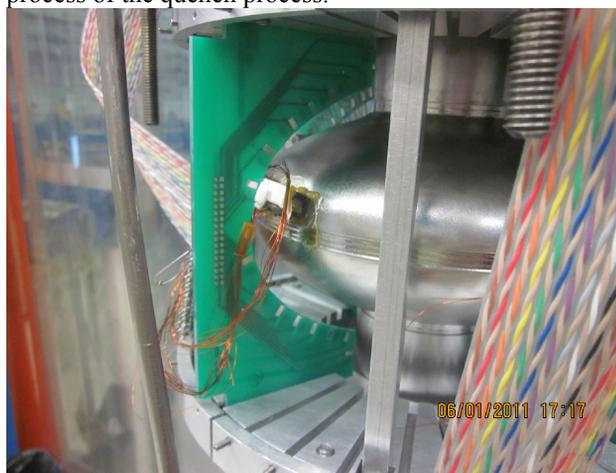
Figure 8: High-resolution local thermometry system developed at JLab for detailed studies of identified defects.
