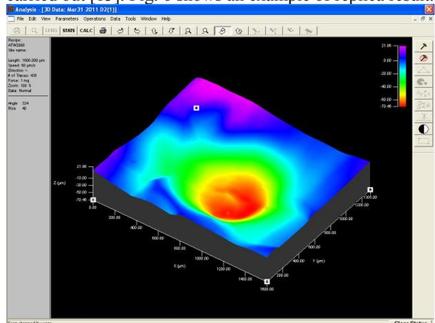
Figure 6: 3D contour of the replica of a defect near the equator weld of a 9-cell cavity.
