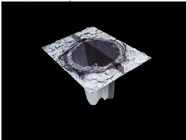
Figure 7: The image of an artificial pit similar to those created on the inner surface of a 1-cell cavity for advanced quench studies.
