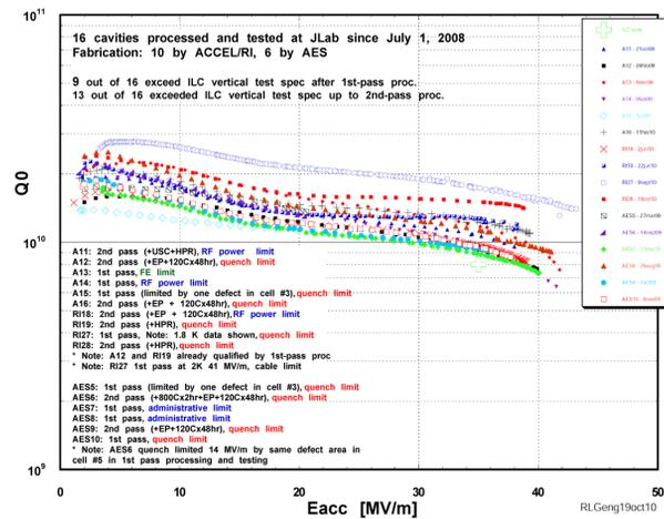
Figure 2:  $Q(E_{acc})$  curves of all baseline 9-cell cavities processed and tested, without bias, since July 2008. Ten cavities are manufactured by ACCEL/RI; six by AES. These cavities are processed up to a second pass. See text for explanation.
