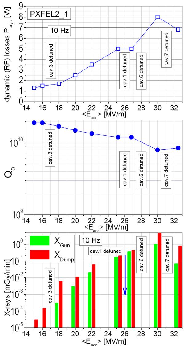
Figure 5: Module PXFEL2\_1 dynamic cryogenic losses, module  $Q_0$  and gamma radiation.
