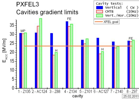
Figure 6: Module PXFEL3 cavities gradients limits (green – single cavities retested after disassembly: H – horizontal cryostat pulsed test, others – vertical cryostat CW test).
