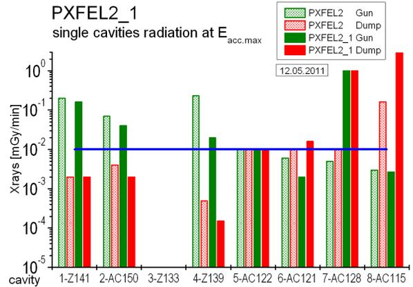
Figure 4: Module PXFEL2\_1 gamma radiation.
