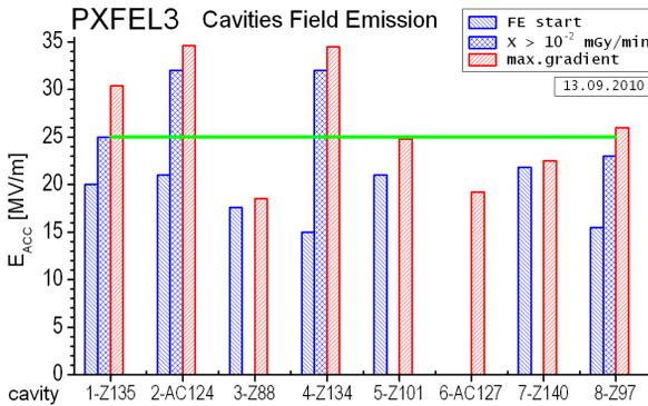
Figure 7: Module PXFEL3 cavities Field Emission onsets compared to maximum gradient.
