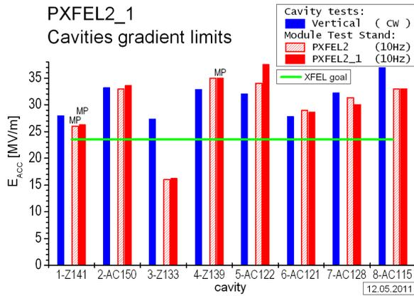
Figure 2: Module PXFEL2\_1 cavities gradient limits.
