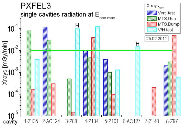
Figure 8: Module PXFEL3 cavities gamma radiation (cyan – single cavities retested after disassembly: H – horizontal cryostat pulsed test, others – vertical cryostat CW test).
