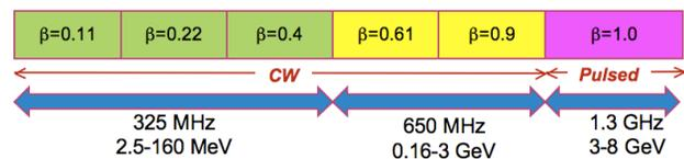
Figure 1: Project X incorporates six types of cryomodules, shown in this map. This paper describes the requirements for 650 MHz, beta = 0.9 cryomodules.
