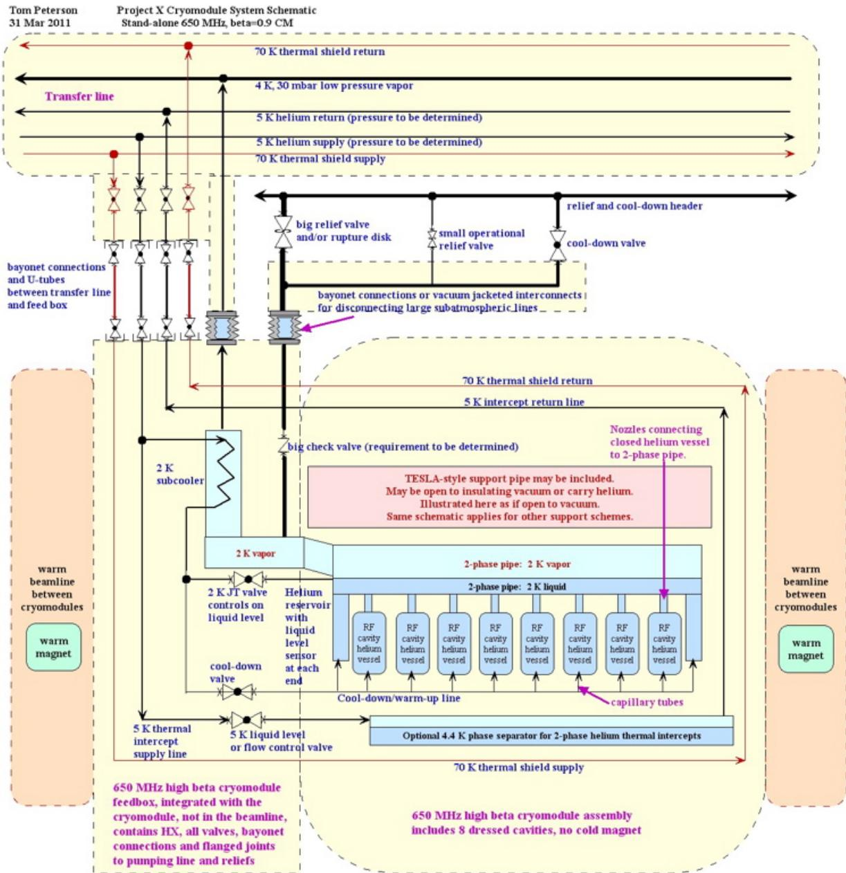
Figure 3: 650 MHz beta = 0.9 cryomodule schematic
