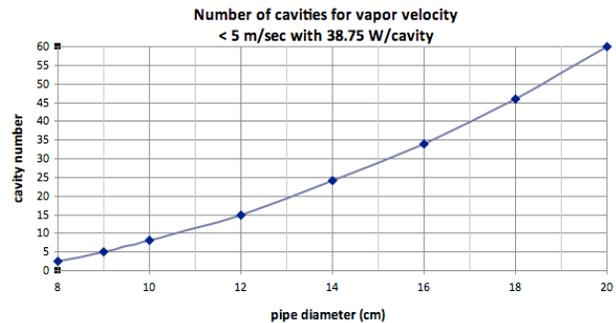
Figure 4: Number of 650 MHz cavities in series, using 1.5 x the estimated heat load shown in Table 1, which results in a vapor flow rate of 5 m/sec versus pipe size.
