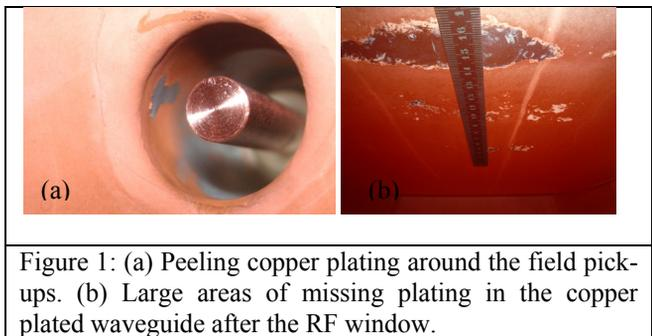
Figure 1: (a) Peeling copper plating around the field pickups. (b) Large areas of missing plating in the copper plated waveguide after the RF window.
