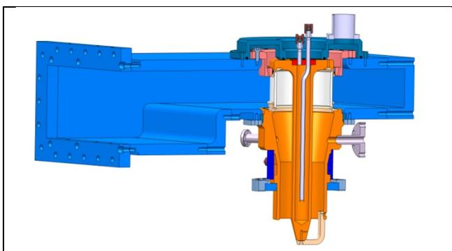
Figure 4: Picture of the new SOLEIL power coupler under development.
