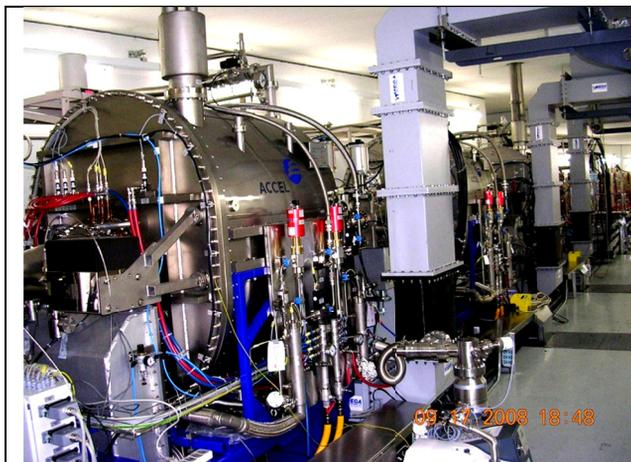
Figure 2: Picture of three installed cavities cryomodules at the SSRF.
