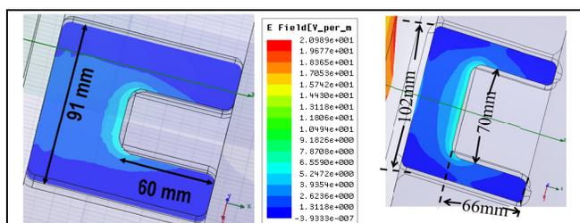
Figure 6. Original Cornell design with  $Q_{ext} = 250k$  (left) and NSLS-II design with  $Q_{ext} = 65k$  (right).
