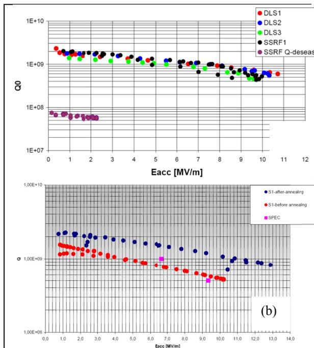
Figure 3: (a) Plot of how the  $Q_0$  degraded on SSRF1 following 10 hrs at a temperature 70 – 130K. (b) Comparison of  $Q_0$  of SSRF1 before and after the high temperature bake
