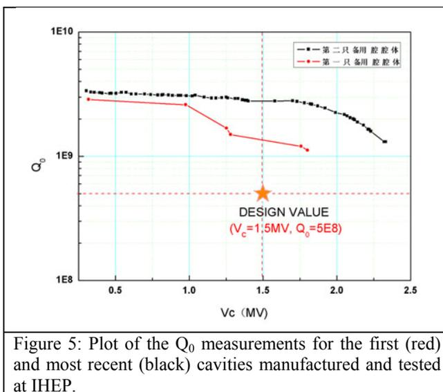
Figure 5: Plot of the  $Q_0$  measurements for the first (red) and most recent (black) cavities manufactured and tested at IHEP.
