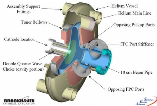
Figure 4: 704 MHz elliptical SRF gun.
