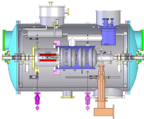
Figure 1: DC-SRF gun at Peking University.
