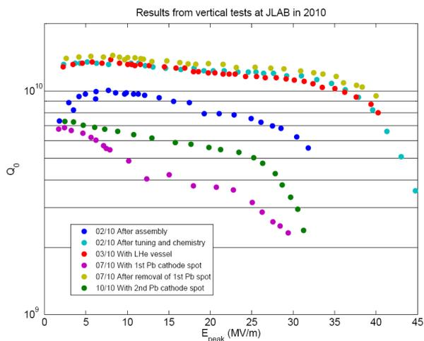
Figure 3: Results of 1½ cell gun cavity vertical testing at Jefferson Lab.
