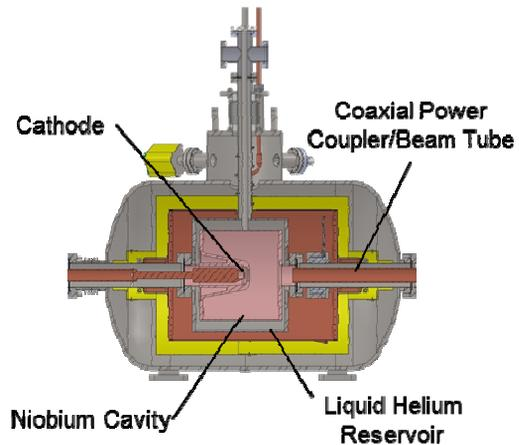
Figure 6: 500 MHz NPS QWR gun.
