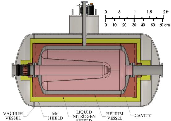
Figure 5: 112 MHz electron gun cryomodule.
