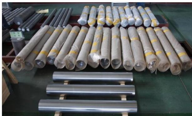
Figure 3: Semi-finished Nb and NbTi products.
