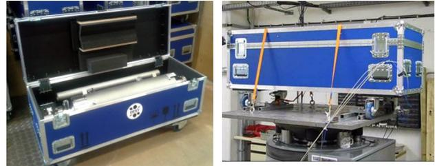
Figure 6: Cavity transport box (left) and set-up for transport test (right).
