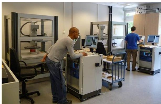
Figure 4: Eddy current scanning of XFEL niobium sheets at DESY.
