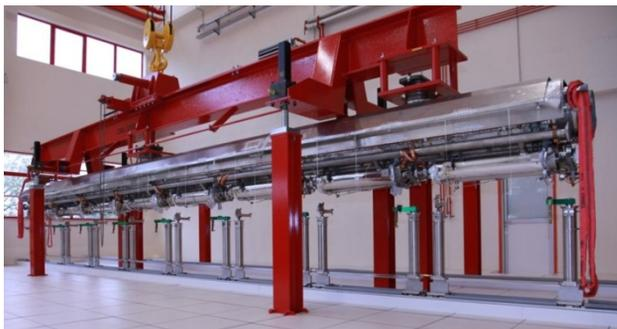
Figure 7: String and module assembly at new CEA Saclay infrastructure.
