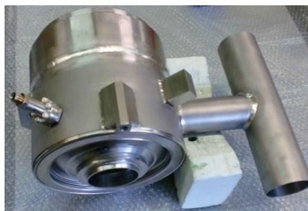
Figure 2: Test piece for weld qualification (Courtesy of RI).
