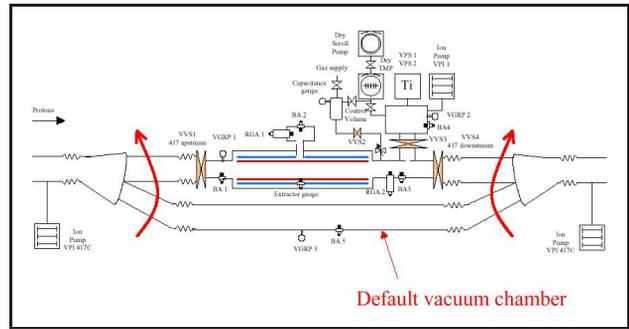
Figure 6: The LSS4 section near the COLDEX region which can host the test crab cavities in the SPS.
