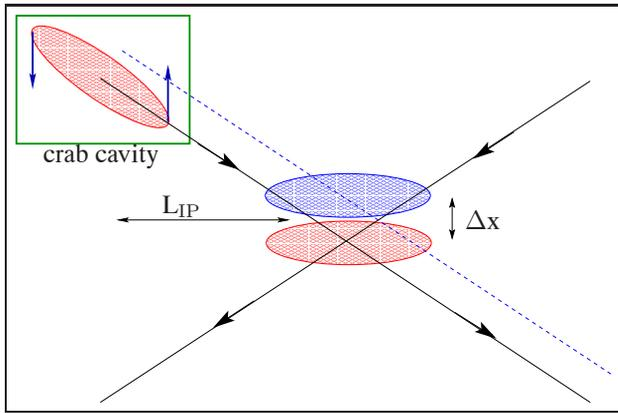
Figure 5: Schematic to illustrate offset collisions due to the crab cavity phase offset w.r.t to the beam. The blue line represents the trajectory of the offset barycenter.
