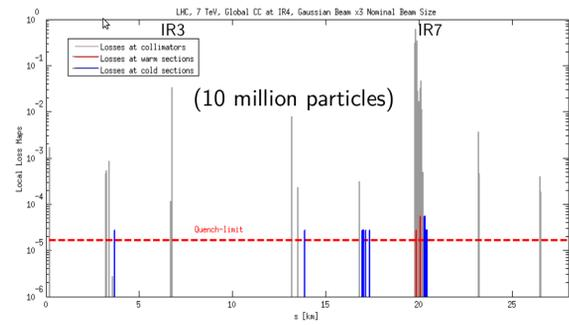
Figure 8: Longitudinal loss map for a particle distribution of  $\times 3$  larger beam size and a 3-turn  $90^\circ$  phase failure with a global crab cavity in the nominal LHC.
