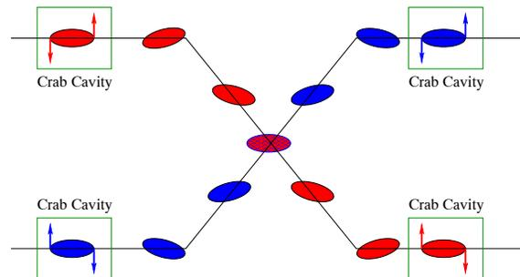
Figure 1: Concept of crab crossing scheme using RF cavities to maximize the bunch overlap at the collision points.
