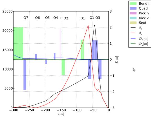
Figure 3: Draft optics and magnetic elements in the IR<sub>1</sub> and IR<sub>5</sub> region for the LHC upgrade with  $\beta^* = 15\text{cm}$  [4]. The pink blocks represent the potential location ( $\sim 10\text{m}$ ) for cavities.
