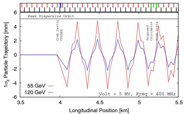
Figure 7: First turn trajectories of a particle at  $1\sigma_z$  near the LSS4 region. Two collimators placed upstream are with the right phase advance to see zero and maximum orbit deviation respectively.
