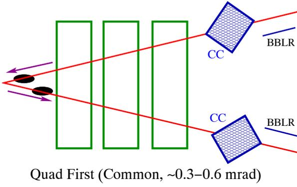
Figure 2: Schematic of the LHC interaction region with common focusing channels and independent crab cavities in a local scheme placed after the beams are separated.
