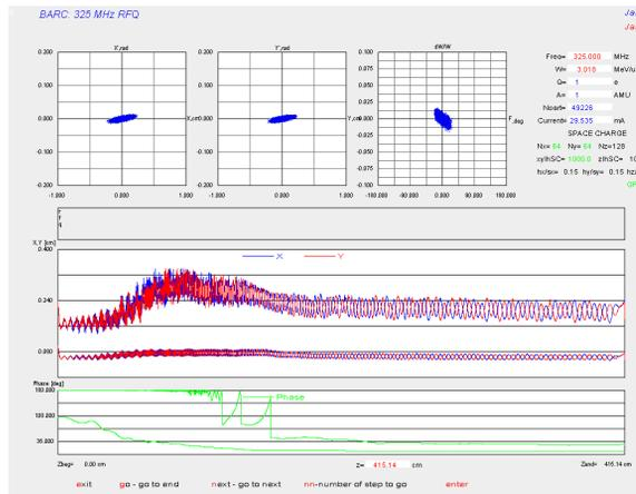
Figure 5: Beam envelop in the RFQ.
