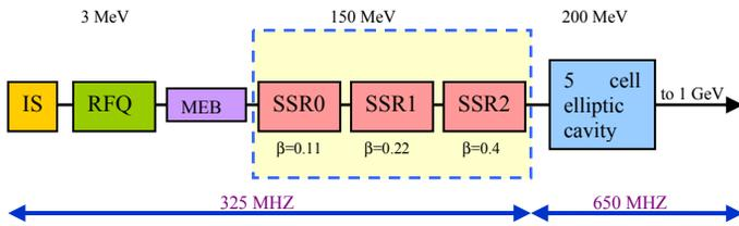
Figure 4: Modified layout of the 1 GeV Linac for ADS.
