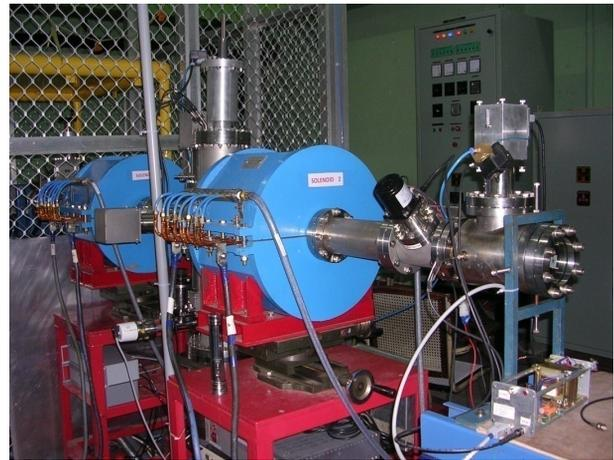
Figure 3: LEBT test bench at BARC.
