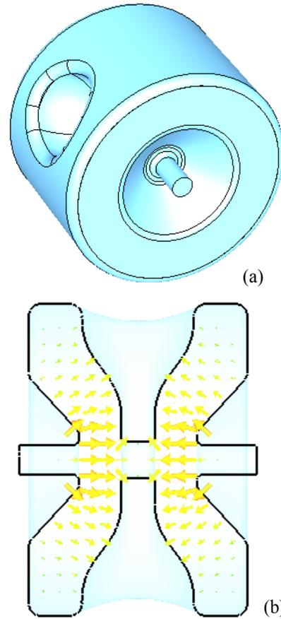
Figure 6: (a) Spoke resonator designed in CST Microwave studio (b) Electric field profile in the spoke resonator.
