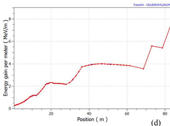
Figure 8: (a) Beam profile along the linac (b) Evolution of emittance along the linac (c) synchronous phase along the linac (d) Energy gain per meter along the linac.
