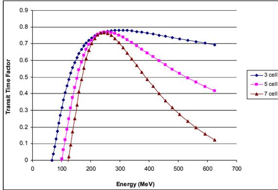
Figure 7: Variation of TTF with energy for different no. of cells/cavity for  $\beta_G = 0.6$ .
