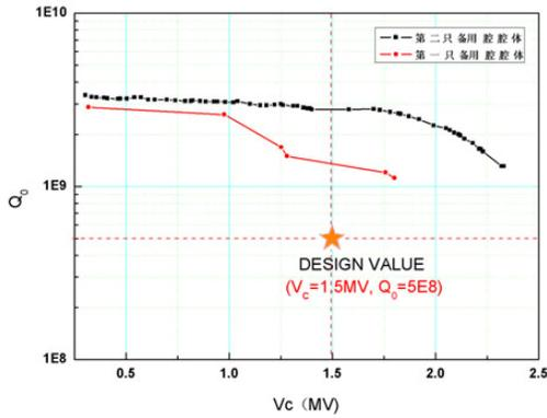
Figure 6: Measured  $Q_0$  on 500 MHz BEPC-II cavity.
