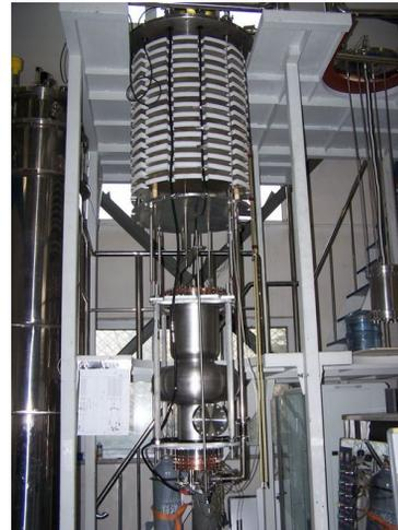
Figure 5: 500 MHz cavity for BEPC-II.
