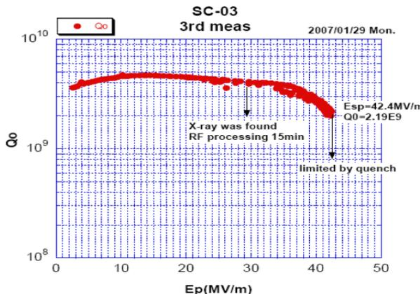
Figure 4: Measured  $Q_0$  of the 1.3 GHz single cell.
