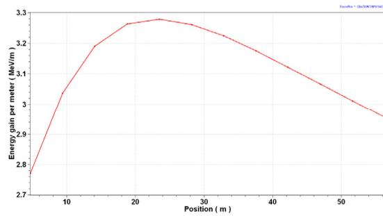
Figure 9: Energy gain of the spoke cavity.
