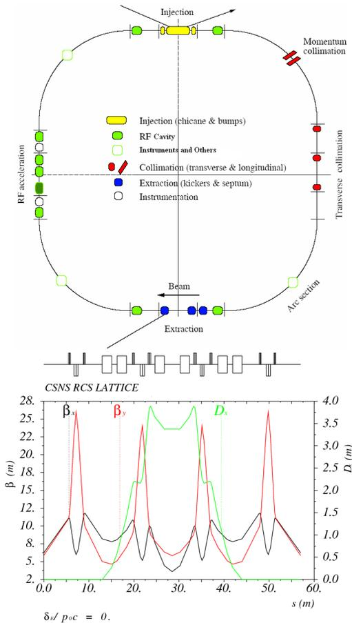
Figure 8: RCS function arrangement(upper) and twiss parameters of one super-period(lower).
