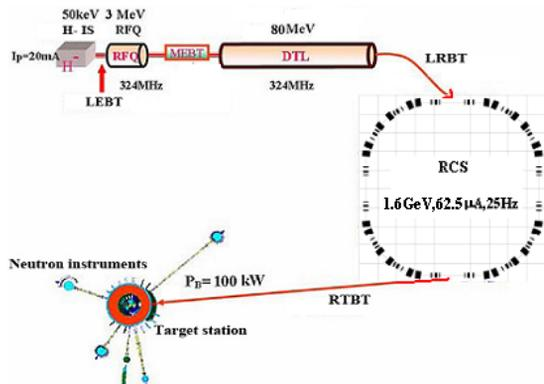
Figure 7: Schematics of the CSNS complex.
