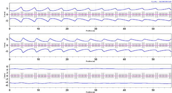
Figure 10: Beam envelopes in three directions simulated.
