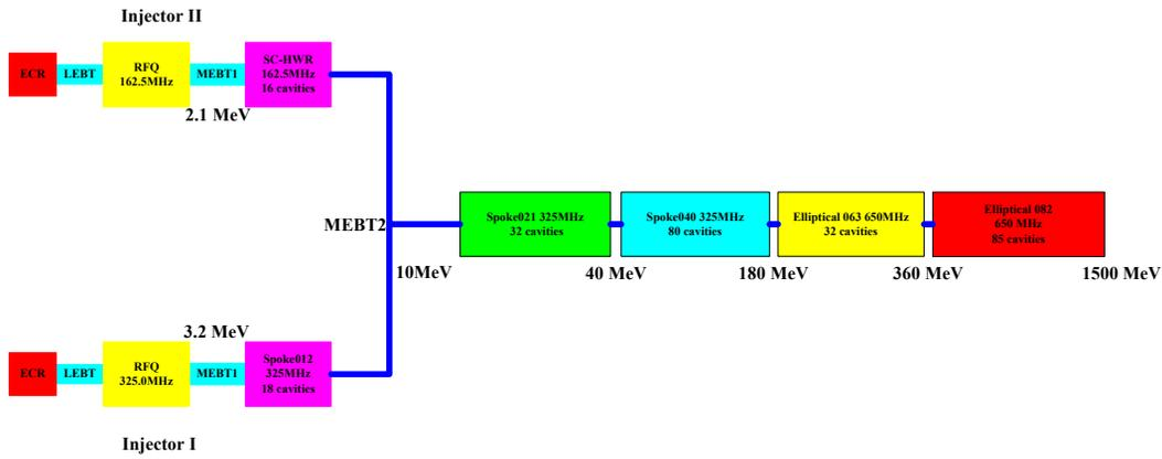
Figure 2: Sketch of the ADS 1.5 GeV linac.
