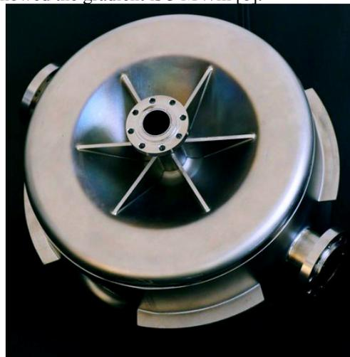
Figure 4: 450 MHz single spoke cavity.
