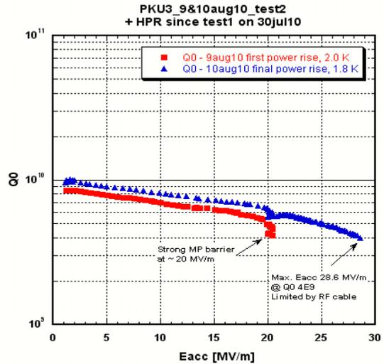
Figure 2: vertical test result of PKU3.
