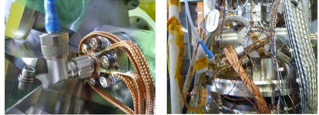
Figure 5: Setup for vertical test of cavity #3. (left) Thermal anchor around HOM pickup connector. (right) Cooling for HOM couplers.
