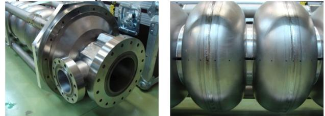
Figure 10: prototype 9-cell cavity #2. (left) titanium end plate for He jacket and flanges and (right) stiffener rings.
