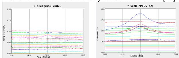
Figure 13: (left) Temperature mapping and (right) X-ray mapping for  $\pi$ -mode at 23 MV/m at the 3rd vertical test of cavity #2.
