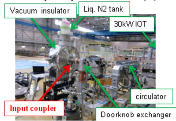
Figure 14: Setup for high power test for input coupler, under 80K temperature
