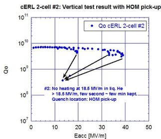
Figure 4: Results of vertical test for cavity #2
