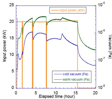
Figure 15: Results of high power test. RF power had been kept to be 20 kW.
