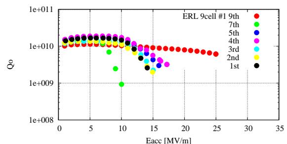
Figure 11; Vertical test results for prototype main linac 9-cell cavity #1.
