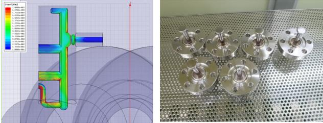
Figure 3: (left) Magnetic field distribution of HOM coupler. (right) Pickup probes for HOM coupler.
