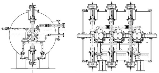
Figure 8: Cryomodule system for injector part.
