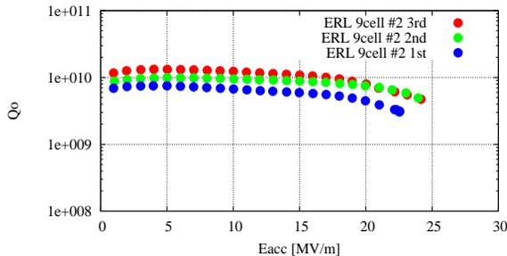
Figure 12: Vertical test results for prototype main linac 9-cell cavity #2.
