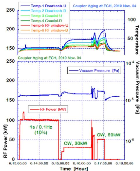
Figure 7: Results of high power tests for prototype input couplers. Plots for (top) temperature and (bottom) for vacuum and RF power.
