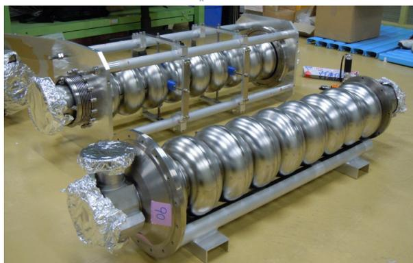
Figure 18: (top) Design of the cERL main linac cryomodule. (bottom) 9-cell cavities, which will be installed into the cERL cryomodule.
