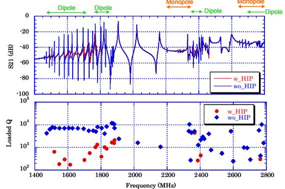
Figure 17: (top) HOM spectrum and (bottom) loaded Q values for with (red) and without (blue) HOM absorber model with HIP ferrite.
