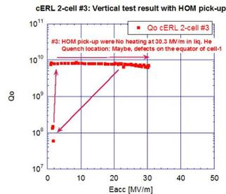
Figure 6: Vertical test results for cavity #3.
