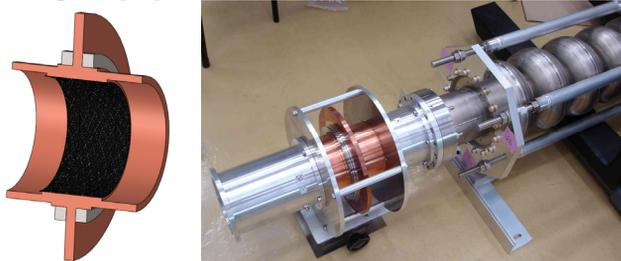
Figure 16: (left) Schematic view of the HOM absorber model with HIP ferrite. (right) The HOM absorber model mounted on the cavity #2 for HOM measurement.
