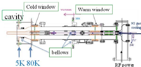
Figure 5: KEK-cERL input coupler for main linac.
