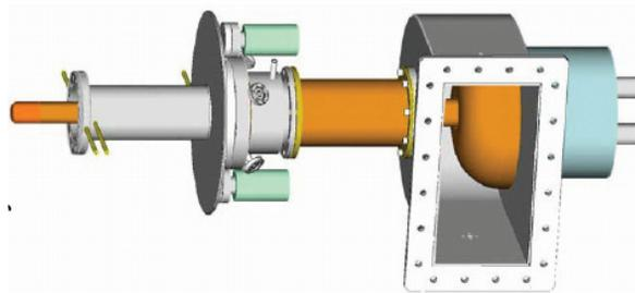
Figure 6: BNL-ERL main linac input coupler.
