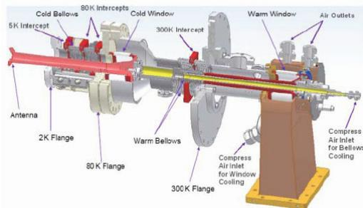
Figure 2: Cornell ERL injector input coupler.
