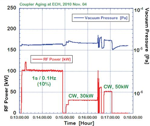
Figure 4: (top) high power test stand, (bottom) results of coupler processing at test stand.
