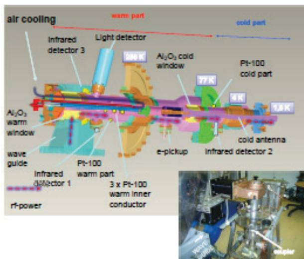
Figure 7: TTF-III coupler test for CW operation at HZB.
