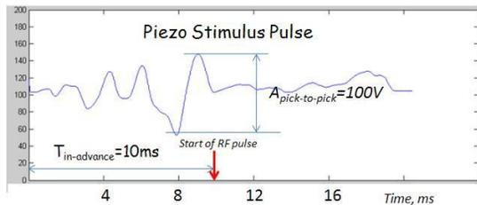
Figure 2: Compensation piezo waveform for a Blade-Tuner equipped nine-cell elliptical cavity
