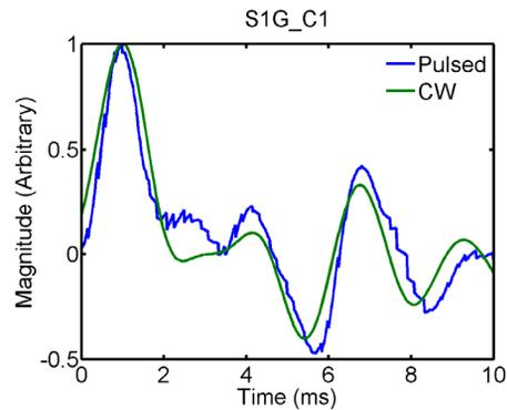
Figure 1: A comparison of the Piezo-Detuning Impulse Response measured during CW and pulsed operation.
