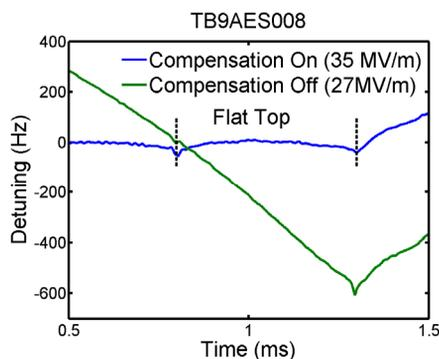
Figure 3: Lorentz force compensation in a Blade-Tuner equipped nine-cell elliptical cavity.
