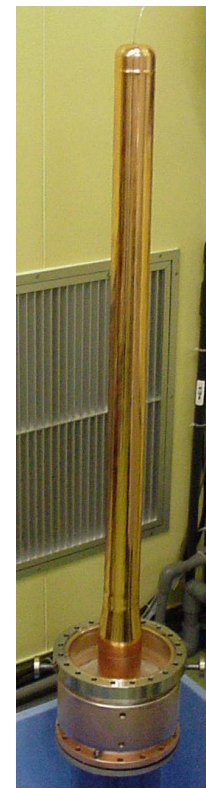
972 MHz Pulsed Coupler for ADS (KEK/JAERI)
