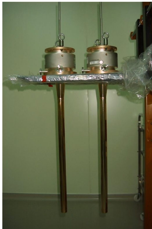
972 MHz Pulsed Coupler for ADS (KEK/JAERI)
