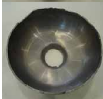
Directly formed from the sliced sheets. No annealed the sheets.
