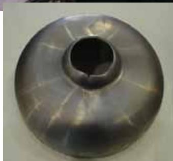
LL End single cell cavity (End cell shape)
