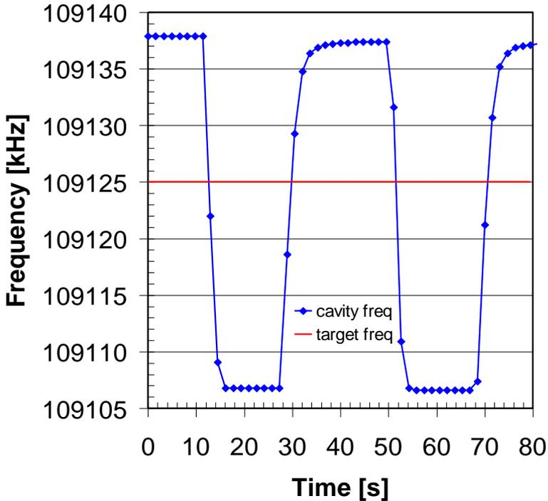
■ 1.2 kHz/s slew rate on-line
