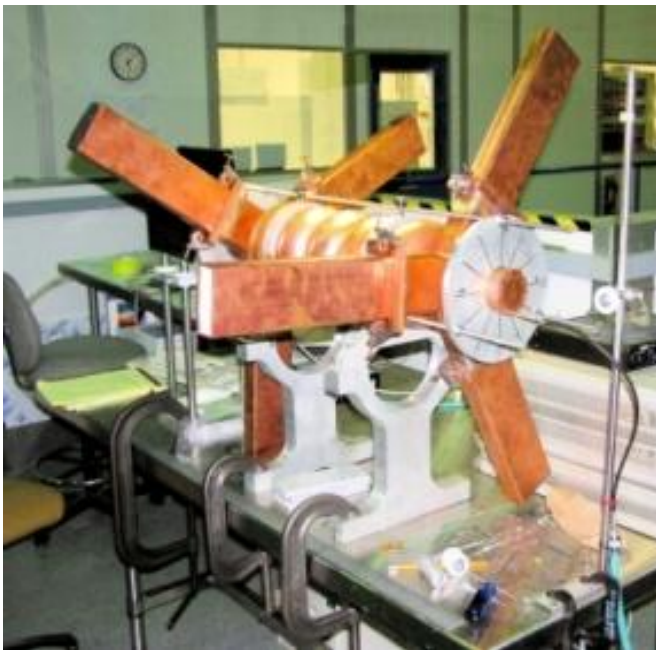
Bead-pull HOM measurement setup
