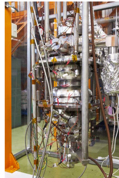
090403 ERL-injector 2cell cavity 2K Keeping at 15 MV/m (CW) E_{acc} and Feed through temp.
