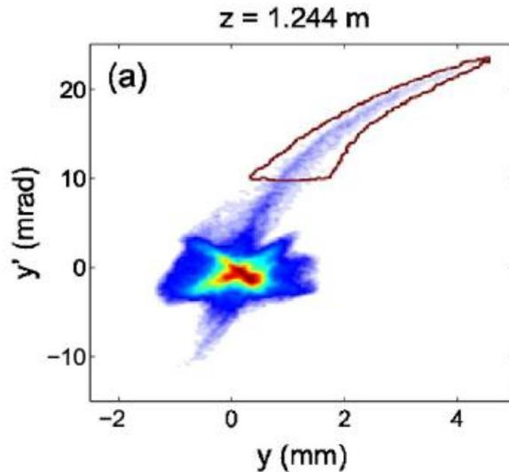
**This Brightness reduction has been traced back to asymmetric photon distributions on the cathode.**
