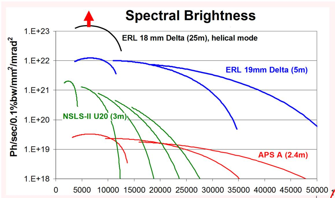
Electron beams from ERLs can have much higher brightness, especially in the core of the beam.
