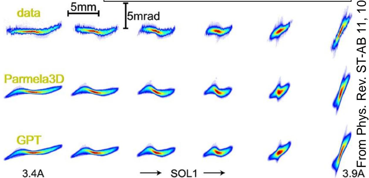
Are transported through the accelerator, measured in a fixed slit phase space measuring system, and compared with simulations.
