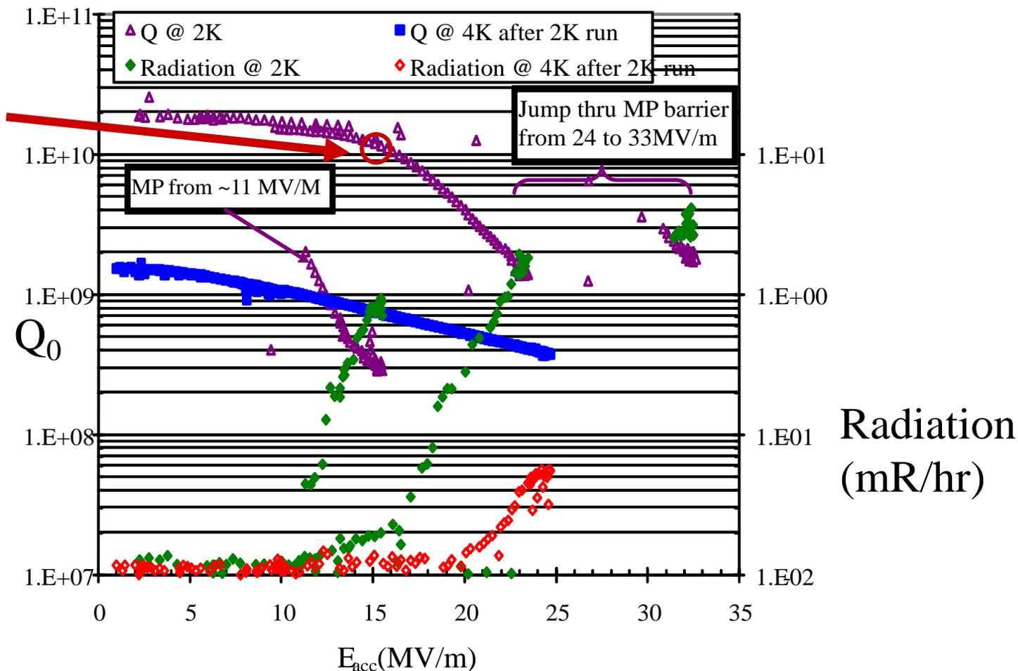
$Q_0$  .vs.  $E_{acc}$  and x-ray intensity as measured at the top of the VTS
