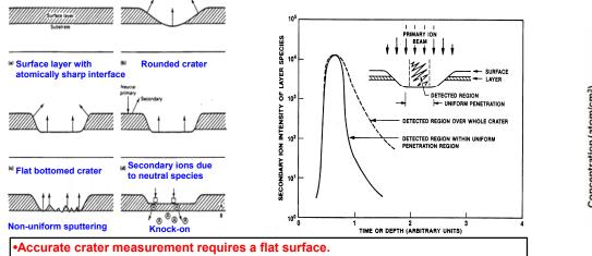
Poor crater shape and rough surfaces will distort profiles (loss of depth resolution). Reduce side-wall contributions by detecting ions from center of larger crater. Optimize distance from wall to detected area
