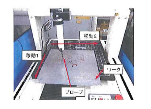
EM/C ET5002A with probe:EPT-4 512kHz, 42dB, 10~220Hz, 63°, lift off 0.5mm, 20mm/s
