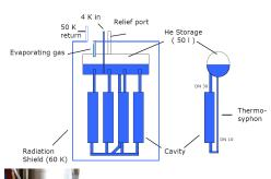
1st cool down successful LHe level reached within 200min Static losses: ~1W
