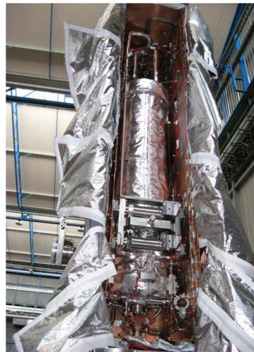
Cryomodule during assembly showing cavity (inside superinsulation), tuning system, thermal shield and outer conductor of the power coupler (at the bottom)
