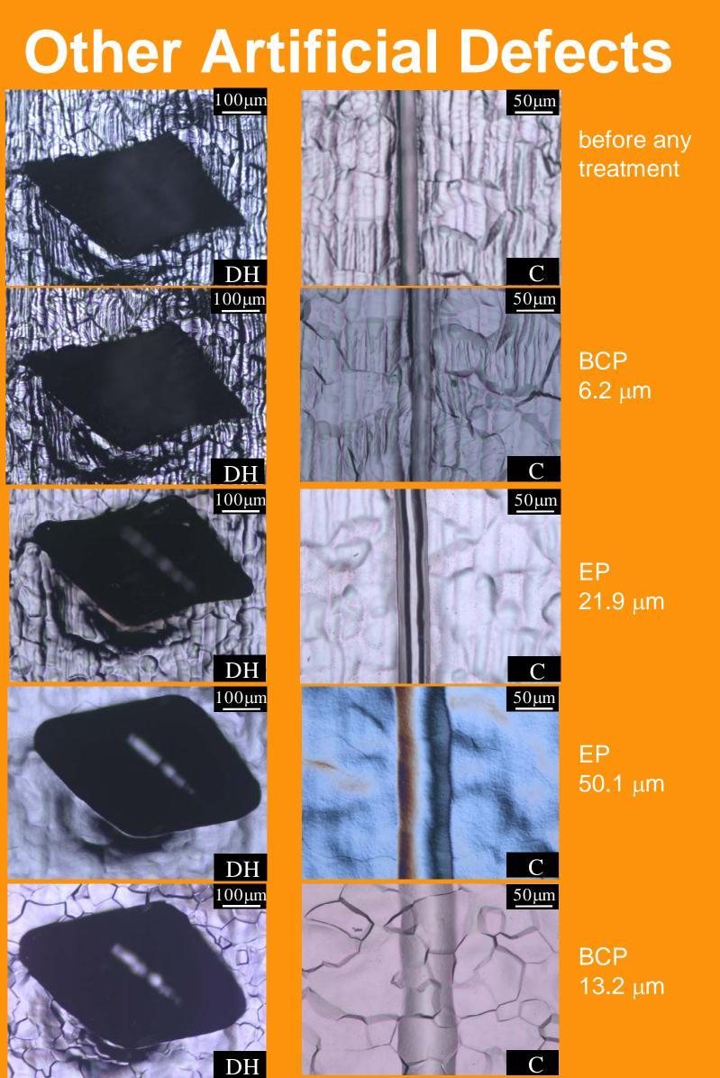
•rhomboid defect (DH) and linear defect (C) evolution during the various steps of the surface etching:
