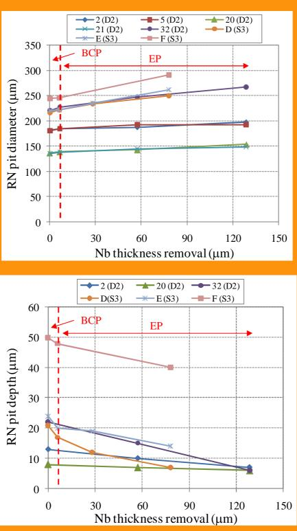
•increase of the pit diameters with the material removal, more enhanced for defects with initial larger diameter
