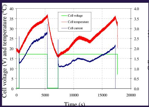
Constant voltage process: 17 V Charge through the cell (C) Typical behavior of the voltage, current and temperature during the EP process
