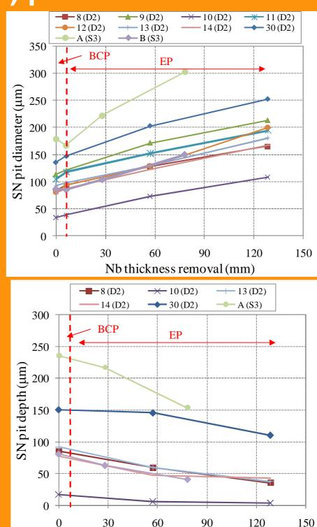
Nb thickness removal (mm)
