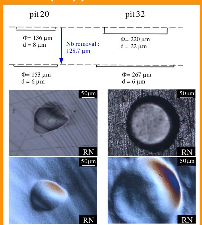
•schematic evolution of RN pits (#20 and #32) and SN pits (pit #10 and pit #30) shapes, after 128.7 μm of Nb removal •all pits change during the decrease of the surface thickness induced by the treatment
