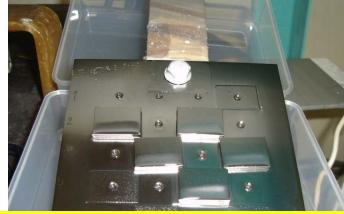
**Exposing the samples to the air for** 30 min. w/o Pure-Water (P.W.) rinse. No stain appeared.
