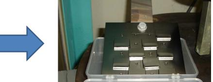
Exposing the samples to the air for 70 min. w/o Pure-Water (P.W.) rinse. No stain appeared.
