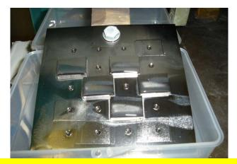
Exposing the samples to the air for 30 min. w/o Pure-Water (P.W.) rinse. No stain appeared.
