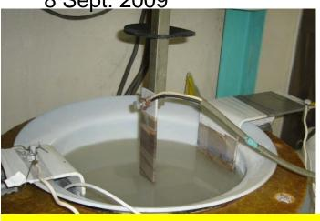
Labo-EP (20 um) with EP acid  $([Nb] = 4.4 \sim 4.8 \text{ g/L}) \text{ at Nomura}$
