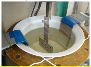
Labo-EP (20 um) with new EP acid ([Nb] = 0 ~ 0.4 g/L) at Nomura
