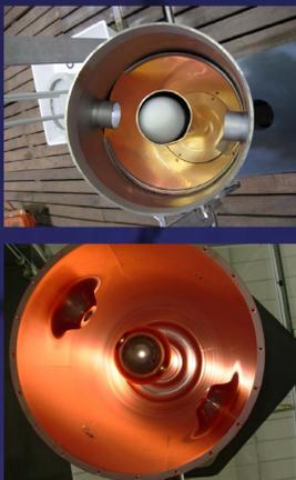
Simulations of the fluid velocity of the SUBU injected into the cavity by four tubes, have shown that the velocity of the fluid close to the bottom wall of the cavity is uniformly distributed: the values obtained vary between 0.04 m/s and 0.06 m/s. Since they are lower than the calculated Reynold number no turbulent motion is expected.
