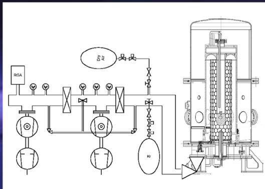
The coating system is designed for Bias Diode Sputtering. Inside a class 10 clean room the cathode-grids structure and the cavity and the vacuum chamber are assembled. The closed chamber is then connected to the pumping system outside the clean room. Cathodes and grids are easily demountable as coating is foreseen for both high  $\beta$  and low  $\beta$  cavities.
