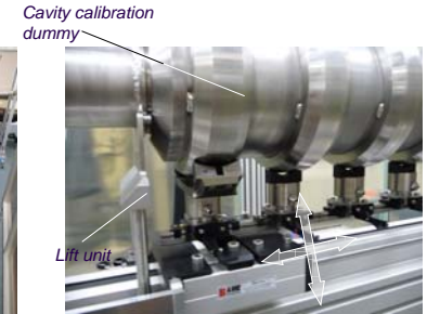
Figure 5. Cavity train with supports and lift unit
