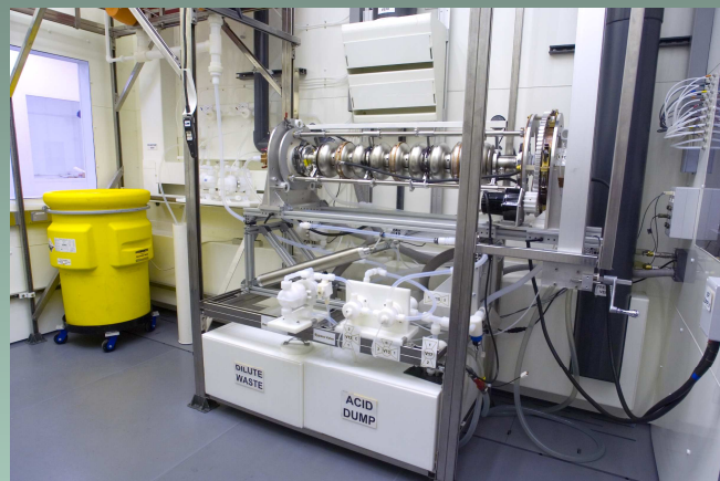
Figure 3. Electropolishing system for 1.3 GHz single and nine-cell elliptical cavities. The system is shown loaded with a nine cell cavity in the horizontal orientation as is the case, for example, during the electropolishing procedure.
