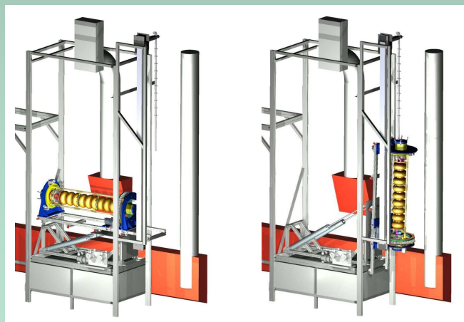
Figure 4. Electropolishing system shown in the horizontal orientation (left panel) as during the procedure and the same system shown rotated into the vertical orientation (right panel) as required for dumping the acid at the end of the procedure and for loading and unloading of the cathode.
