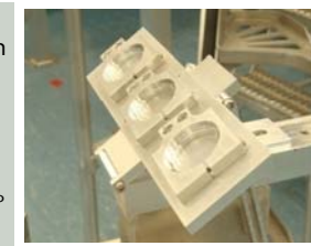
Fixture for holding three samples during HPR
