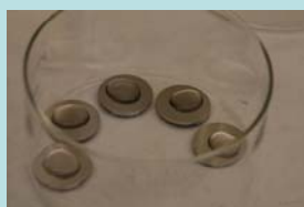
Five niobium samples with 0.5 ml particulate/water suspension drying in cleanroom air
