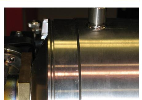
The main coupler is aligned in the horizontal position and parallel to the moving cart using a bracket that engages the coupler flange. The helium vessel is mounted to the cart supported by the bearing lugs and travels along a rail track with bearing rollers. This fixture enables us to adjust and achieve the cavity coupler flange to the helium vessel lugs perpendicularity requirement.
