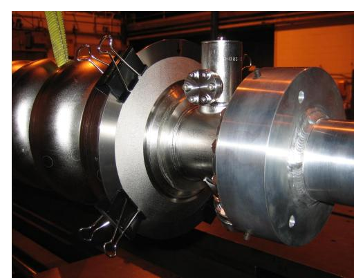
Titanium transition rings are electron-beam welded to the niobium/titanium conical end disks. They are welded from both sides to fully consume the joint for compliance to ASME Boiler & Pressure Vessel Code. Shown below is the joint configuration before and after welding.
