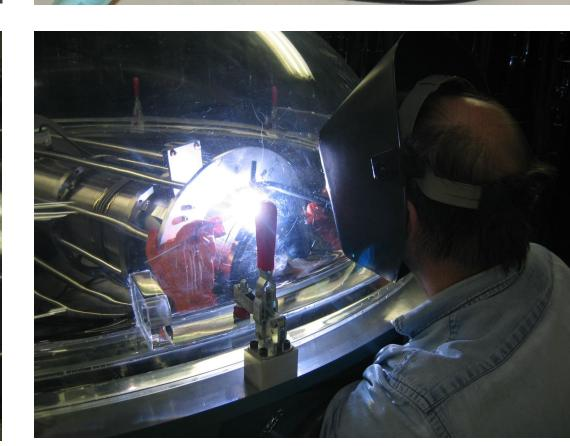
The TIG welding done inside the glove box is operating on three separate argon purge lines. One line is dedicated for the dome purge; a second line has a purge flow inside the helium vessel and the third line is for torch purge and torch cooling. The cables for monitoring the frequency spectrum of the cavity are also attached and connect to feedthrough ports inside the glove box. Once the oxygen level is below 20ppm and humidity levels below 15% are achieved, welding can begin.
