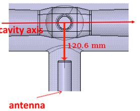
The distance  $\lambda/4 = 430$  mm must be avoided for the distance between ceramic and cavity because it corresponds to a maximum of field in the ceramic in SW
