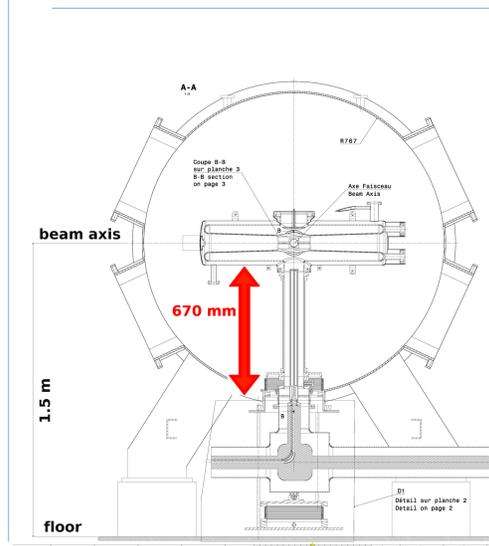
The coupler has to fit under the cavity and the beam axis is fixed at 1.5m from the floor
