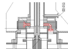
The implementation of a **biasing system** against multipactor will be possible for the future IFMIF linac with a modification of the the design of the transition box
