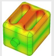
Surface electric field (left) and magnetic field (right) of 800 MHz crabbing cavity
